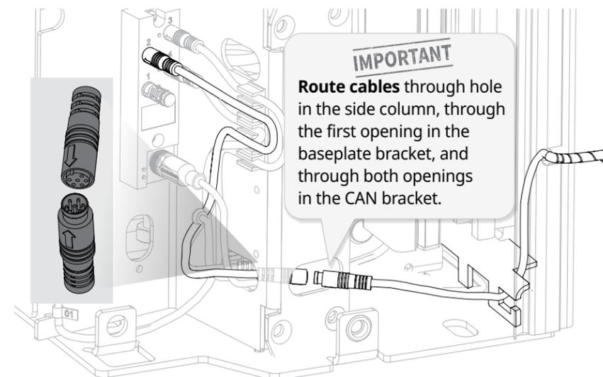
2 Reinstall the CAN bus brackets in both side columns.
