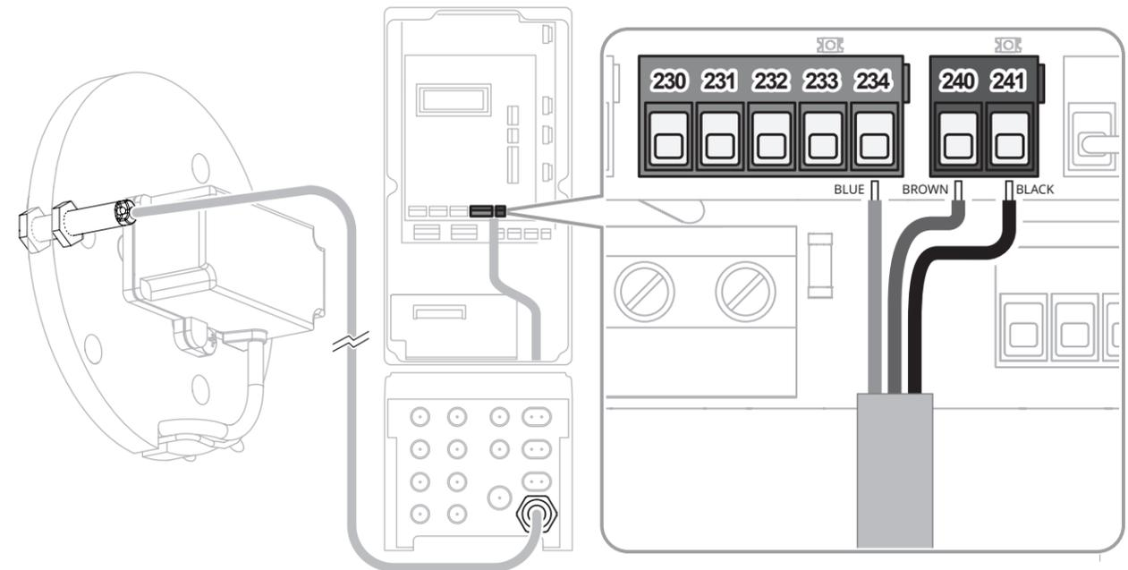
**3** Connect the wiring from the encoder.
