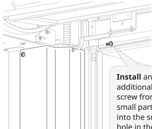
Install an additional screw from the small parts box into the screw hole in the corner bracket.
