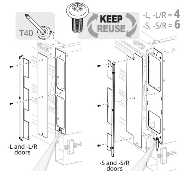
**IMPORTANT** The screw that secures the mounting cradle is preinstalled behind the cover and bracket.
