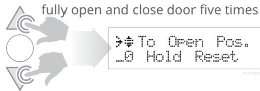
Press and hold the arrows to fully open, then fully close the door five (5) times.
