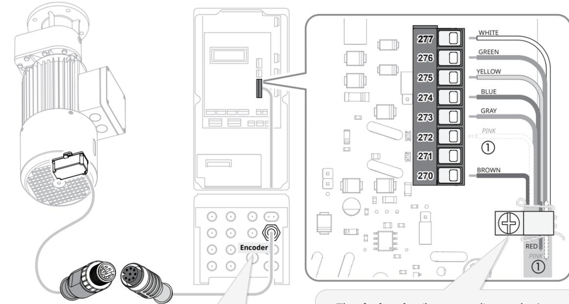
Mark controller end of cable as "Encoder"
