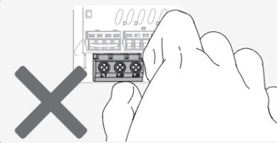
**Do not** try to remove the green terminal block from the circuit board.
