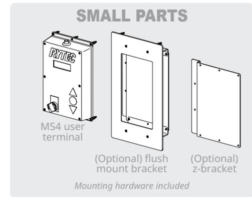
**2** Anchor the user terminal at an easily accessible height using the included hardware. The user terminal can be mounted onto the wall, flush to the wall using the optional bracket, or onto the side column using the optional z-bracket.
