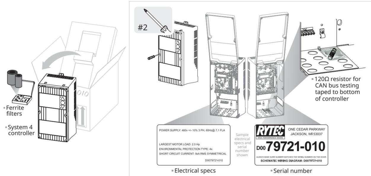
**Verify** that the serial number and electrical specs for the controller match the door.
