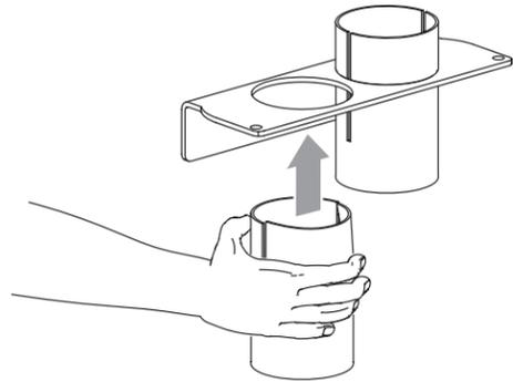
**3** **Install** the bracket into the side column.
