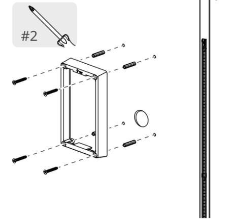
**4** For side column mounting, **install** the grommet into the cable access hole.
