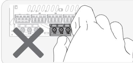
Do not try to remove the green terminal block from the circuit board.
