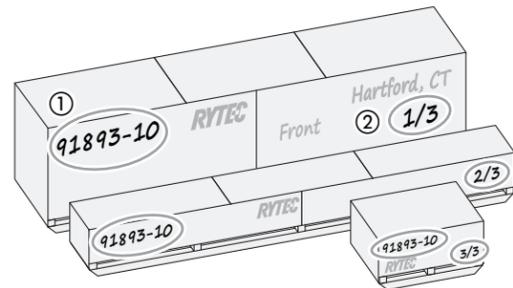
Mixing parts from different doors voids the warranty for all doors in the installation.
