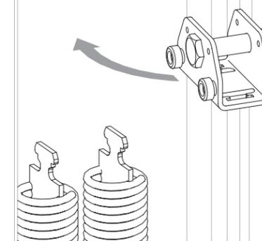
**10** **Loop the spring strap** around the bolt in the spring bracket.
