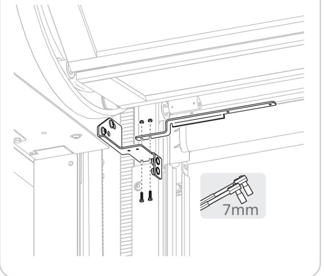
**6** Reach into the drive side compartment and **remove** the wireless antenna and antenna bracket from the top of the motor.
