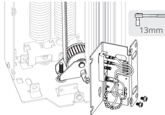
**2** Loosen the top nut of the bolt on the side opposite to the side the belt favors.
