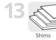
If necessary, shim the side columns so they are plumb to each other.
