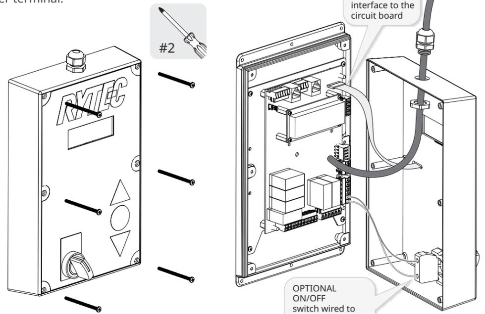
**3** Trim jacket on M8 flying lead to expose wires, and **connect** wires to terminals 380-383.
