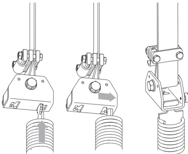
**15 Stretch** the springs downward. **Slide** the bottom spring tabs into the wide slot ①, through the narrow ②, then **pull up to lock** it into the retaining slot ③.
