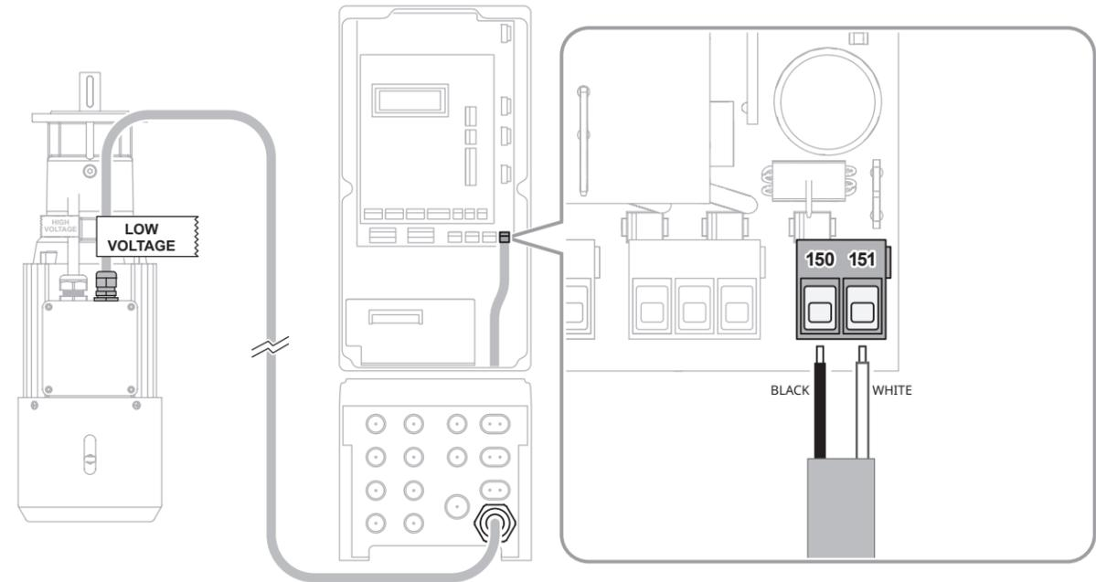
**2** Connect the wires from the proximity sensor.
