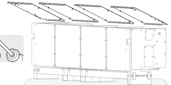
If the door has a preinstalled flat top hood cover, **reinstall** the top panels.
