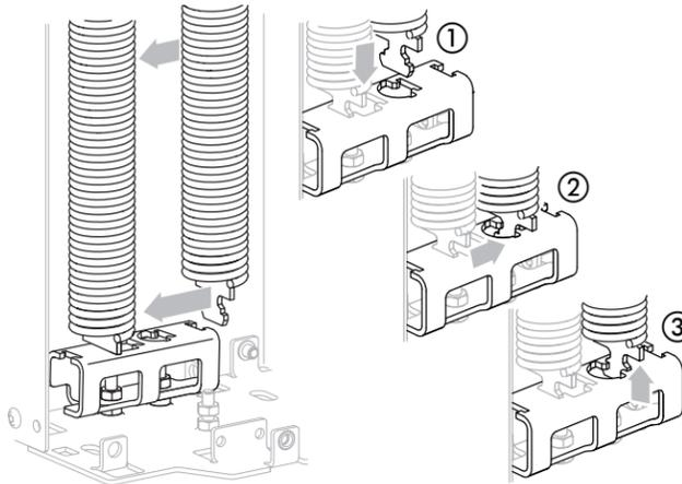
**6** **Make sure** the number of wraps for the spring strap matches the object list ①. **Look through** the front of the console or temporarily **remove** the top access cover.
