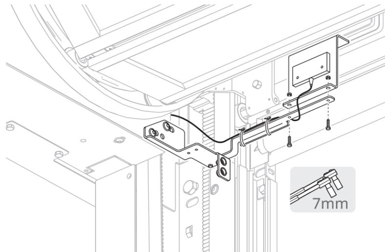
**8** **-US and -US/R doors only:** route the cable to the wireless antenna around the side column and through the gap between the drive side console and the side column.
