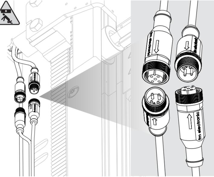
**2** Inside the **non-drive side console**, **connect** the M12 CAN connectors:
