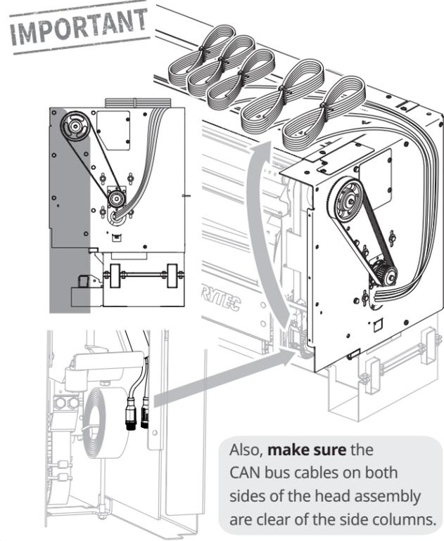
**7** **Remove** the five preinstalled side column screws (located in the shaded area). **Do this** on both sides of the head assembly.
