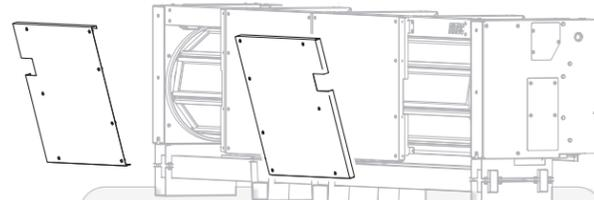
If the door has a preinstalled front hood cover, **reinstall** the front panels. **Locate** the display covers and hardware in the small parts box and **install**.
