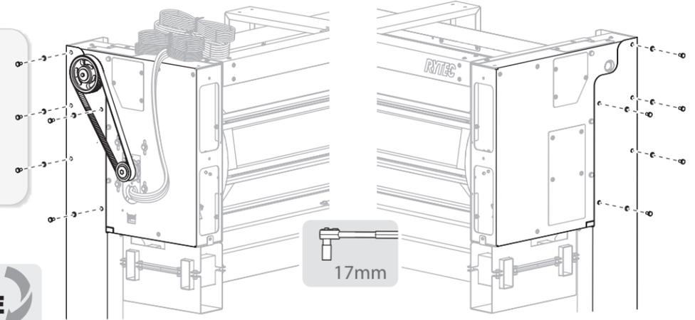
**5** **-S and -S/R doors only:** loosen the screws on the wall mount brackets.
