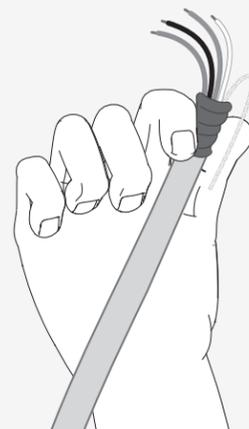
The shield (braided copper mesh) and drain wire (bare metal) must be in contact with the P-clip.
