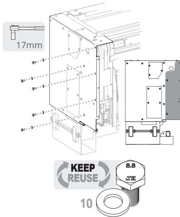
**9** **-S and -S/R doors only:** look for the wall mount brackets at the top rear corners of the head assembly. **Remove** the screws and washers and **flip** each bracket so the flange points up. **Line up** bracket with the rear of the head assembly, then **reinstall** the screws and washers.
