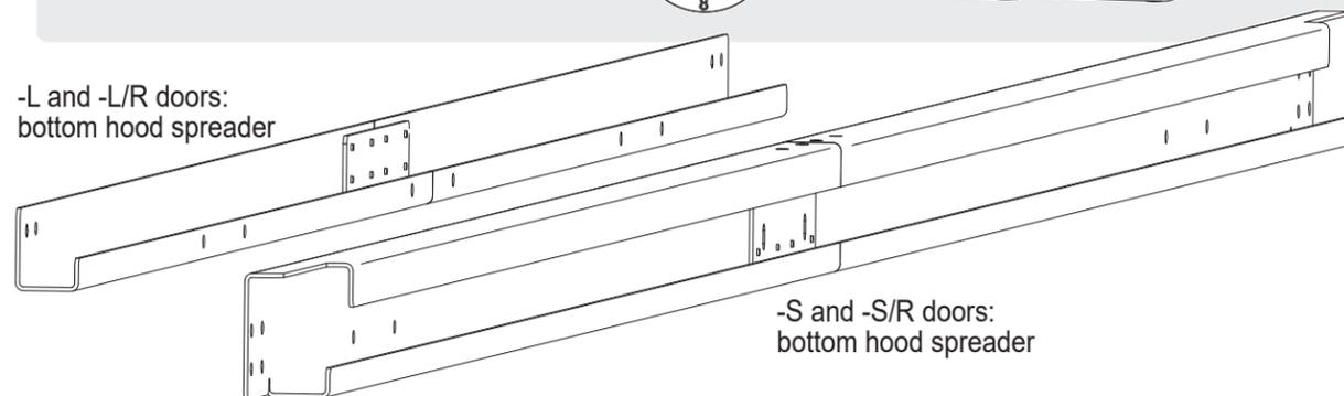
**3** **Attach** the spreader brackets to the bottom hood spreader.
