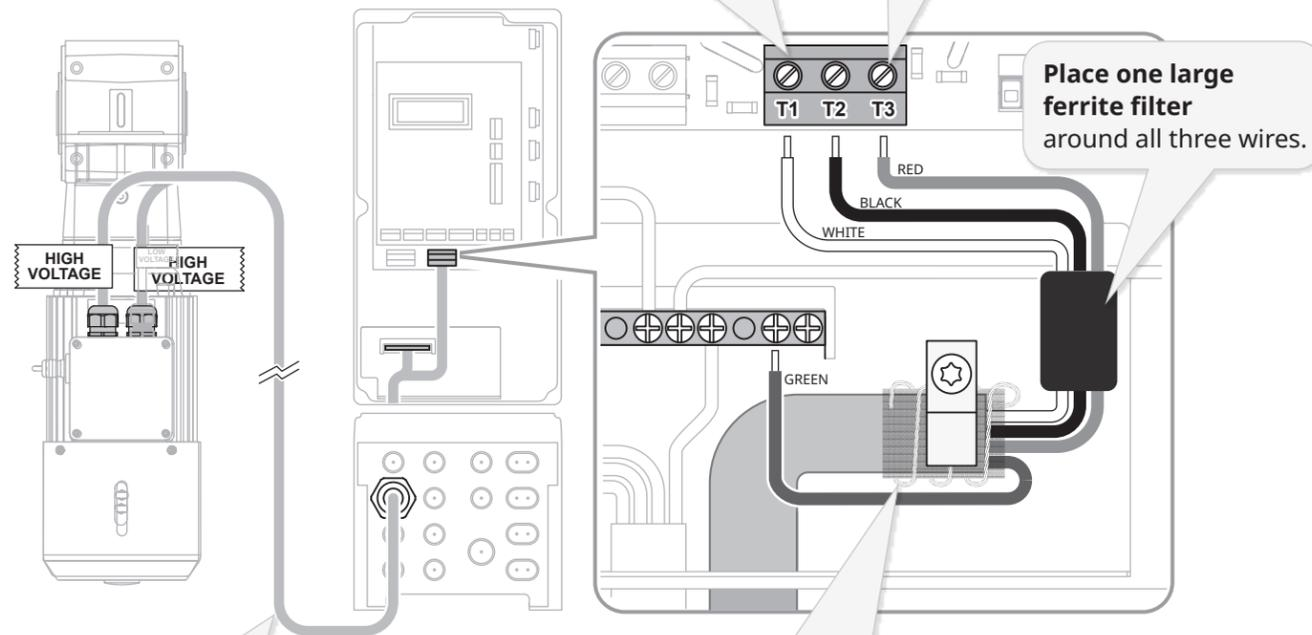
Maximum wire length between motor and controller: 100' (one hundred feet).
