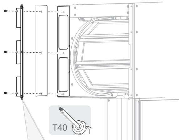
If the door has a preinstalled front hood cover, **reinstall** the front spacer brackets in front of the console covers.
