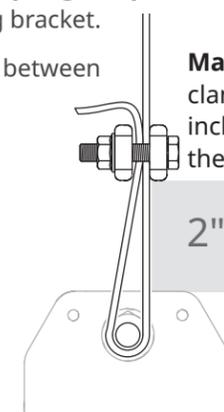
**11** **Set the spring tension.** This is the distance the springs must be stretched to provide the correct tension for the door.
