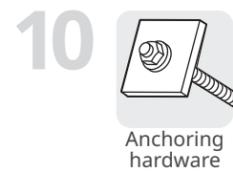
**Anchor** the second side column to the wall at the **top of the side column** and **baseplate**. **DO NOT SET ANCHORS TIGHT** until you have squared the door.
