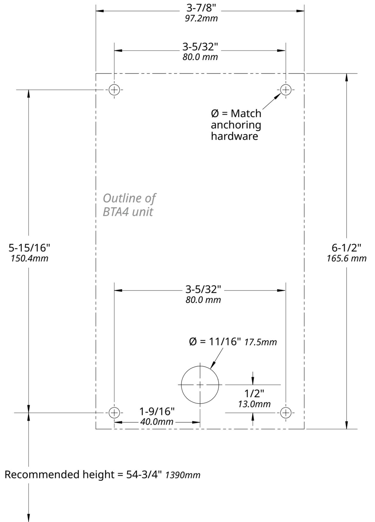
**3** Install the BTA4 frame using the supplied hardware for wall mounting, or your own.
