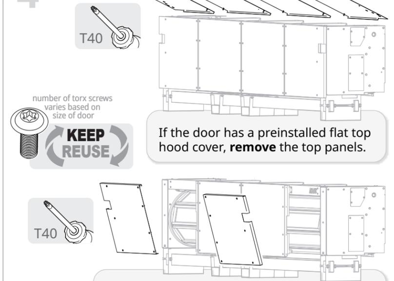
If the door has a preinstalled flat top hood cover, **remove** the top panels.
