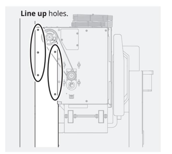
**4** **Secure** the head assembly to the side columns.
