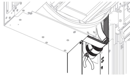
**8** **Loosen the clamp** on the spring strap.
