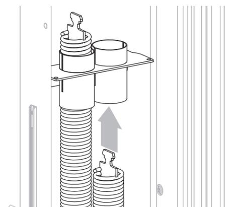
**5** **Slide** the bottom spring tabs into the wide slot ①, through the narrow ②, then **pull up** into the retaining slot ③. The spring should remain upright.
