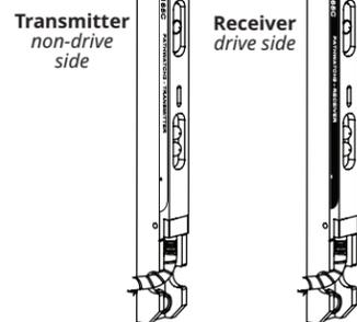
2 Install the jamb mounted SmartSurround™ light curtains and cables onto the drive side and non-drive side walls of the door opening.
