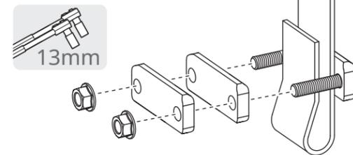
**9** **Position** the spring bracket so that the bumpers and locking tab face the side wall.
