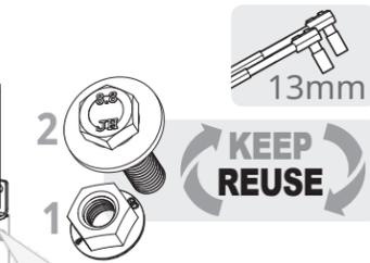
**Use hardware** saved in Step 10 on page 6. Rear screw connects to **flanged nut**. Front screw connects to **riveted nut**.
