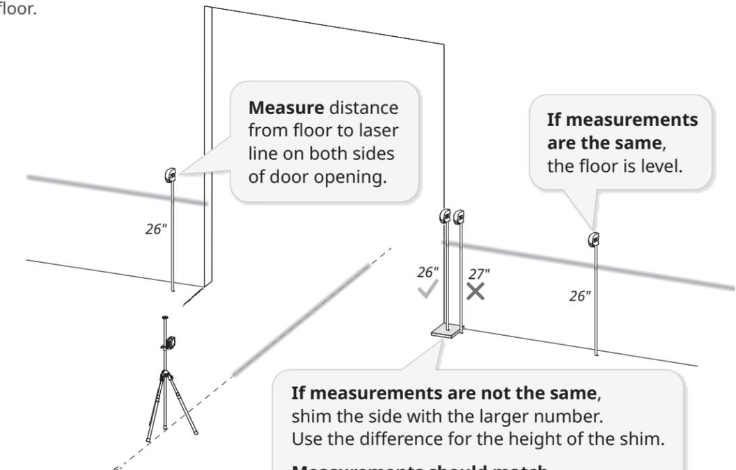
**Measure** distance from floor to laser line on both sides of door opening.
