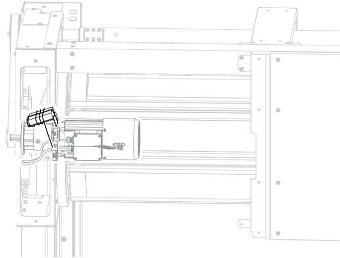
**7** Install the wireless antenna bracket onto the arm.
