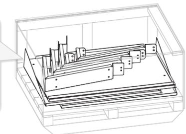
**Bottom hood cover (optional):** panels are crated in front of head assembly, and brackets are crated under the lifting cradle.
