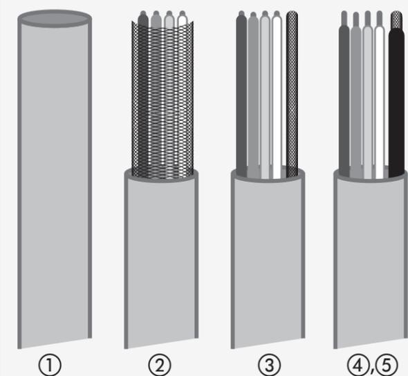
The **shielding** (braided wire mesh) is used as a fifth "wire" and plugs into terminal SH.
