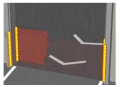
Recognizes when weather elements (rain/ snow/ice) block beams for prolonged period and closes door slowly. Minimizes door open time during these events as long as all other safeties are clear.
