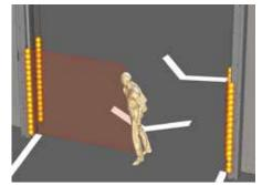
Reduced door opening/closing speed if beams are blocked, or abnormal traffic patterns or unusual doorway presence is detected.
