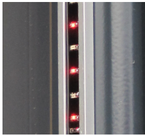
Red lights illuminate to indicate door is closing
